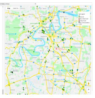
Aldridge's suite of TC1783 flashing school zone sign products are designed to be monitored remotely with software, developed by Aldridge and customised for this product, that is accessible through a secure web portal. So wherever there is internet connection, the signs can be monitored in near real time. It is used for fault reporting, trouble shooting from event log histories and pre-emptive calendar updating.
